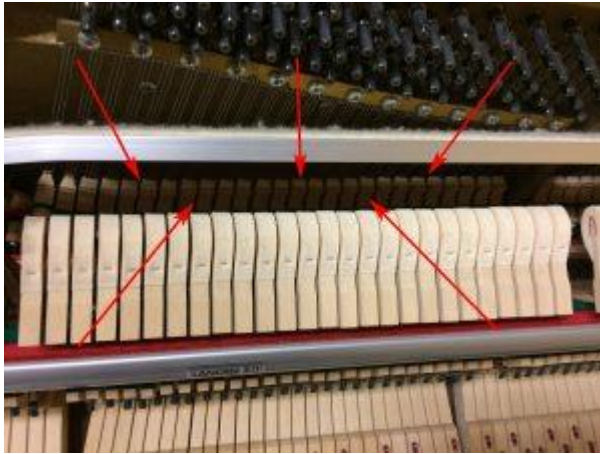
The dampers of an upright piano
